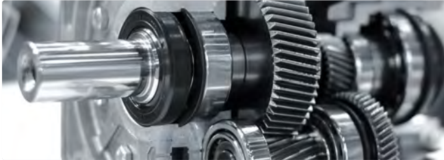
Transmission shaft bearings
